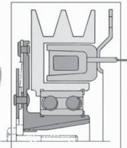
Electric clutches provide for remote control of the feed and chopping mechanisms on straw choppers, insulation blowers, and salt spreaders.
