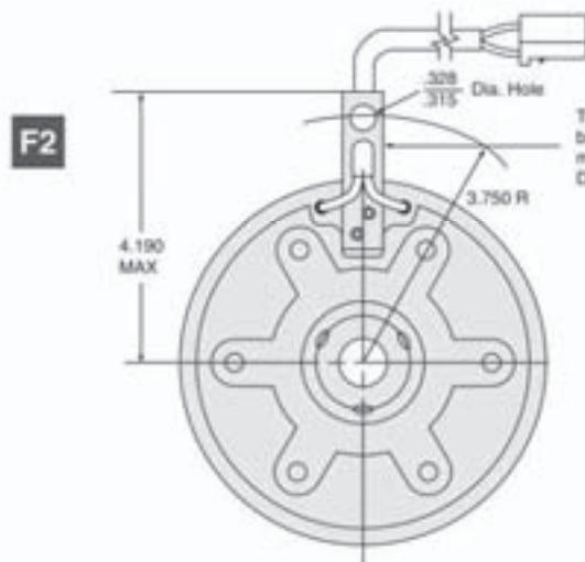
Typical antirotation tang to be loosely pinned to a member to prevent rotation. Do not bolt rigidly.
