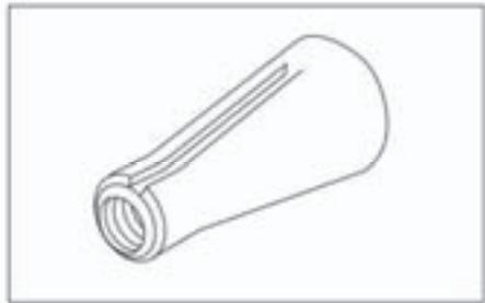
**Tapered bore (4:1)** - shaft tapers three inches per foot, for end of shaft mounting.
