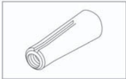
**Tapered bore (8:1)** - shaft tapers  $1\frac{1}{8}$  inches per foot, for end of shaft mounting.
